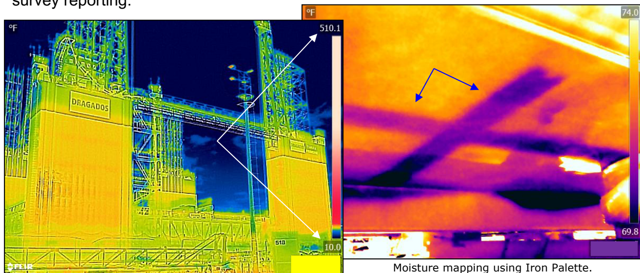
This solar loaded image in Rainbow Palette exhibits poor thermal tuning.
